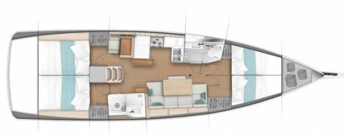
shipyard: **JENNEAU** engine 57 HP launched: It. 200 2023 fuel tank length over all: 13.00 m drinking water tank: It. 530 length of the hull: 12.64 m 8 + 2berths: width: 4.26 m cabins 4 1.60 m draft: salon: convertible
